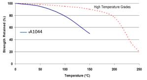
"Hot strength" shear strength tests performed on mild steel. 24hr cure at room temperature and conditioned to pull temperature for 30 minutes before testing.
